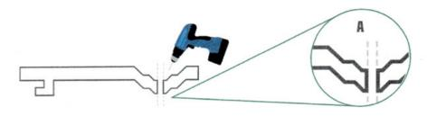
Pre-dill a hole 4.5mm on the panel's rail A position first.
